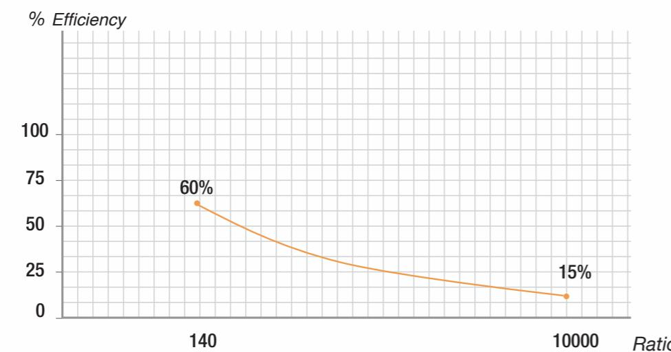
**Rendimento riduttori a ingranaggi / Helical, Bevel and Planetary gearboxes efficiency****A, P, CAM
